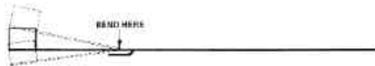
[Figure 4-6. RHODES Damper Arm - Alignment Adjustment](#)
